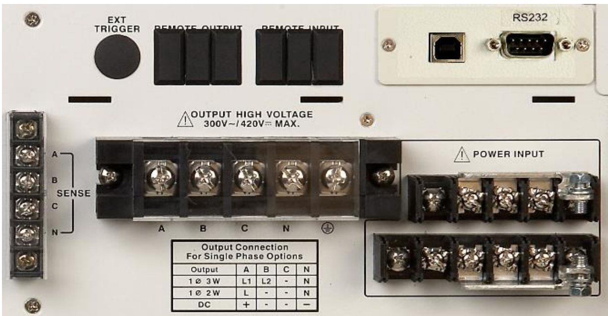
Figure 1: Input/Output Terminal Block and Output Connection Description
